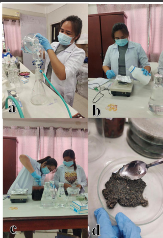
Plate 2: Sample Preparation: (a) Filtration of Distilled Water, (b) Chemical Weighing, (c) Sample Preparation, and (d) Sediment Drying For Analysis
