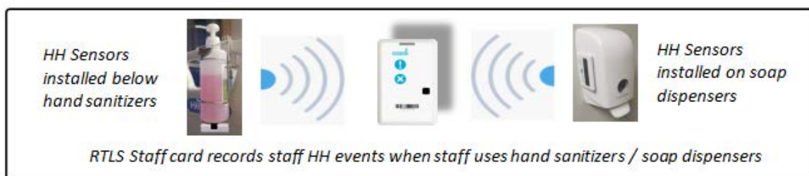
Figure 2: The Electronic Hand Hygiene (Hh) Monitoring System Records Hh Performed by Staff by Recording Interaction Between the Rtls Staff Card Worn by Staff (Middle Picture) With Sensors Installed at Hand Sanitizers (Far Left Picture) And Soap Dispensers (far right picture).
