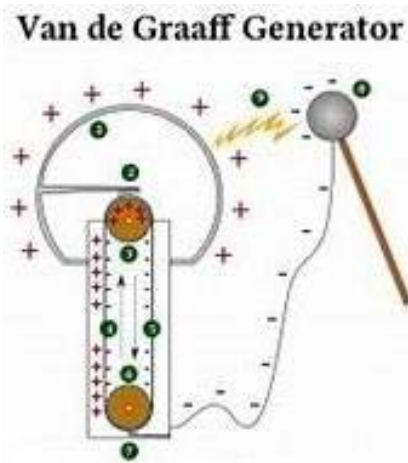
Figure 8: Van de Graaff generator is an electrostatic generator, which uses a moving belt to accumulate electric charge on a hollow metal globe on the top of an insulated column, creating very high electric potentials. The generator was originally developed as a particle accelerator for physics research, as its high potential can be used to accelerate subatomic particles to great speeds in an evacuated tube.
