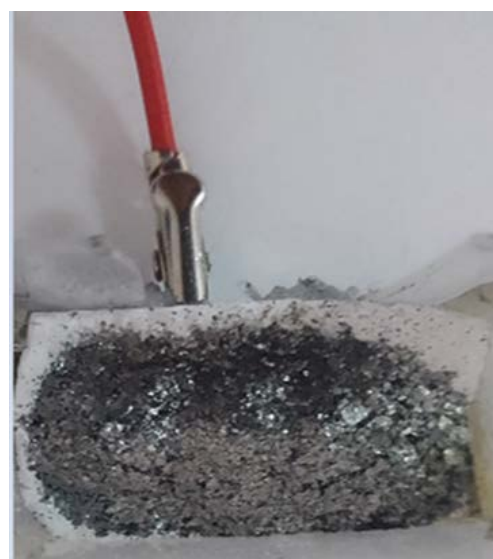
Figure 2: The prepared Al-Air Battery.
